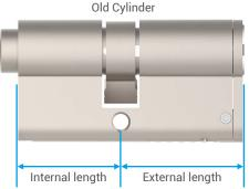
3. Adjust the external side: if external length of old cylinder is no more than 32.5mm, you do not need to do anything. If it is more than 32.5mm, please add the external extensions together to form the difference between 32.5mm and your old cylinder external length.
